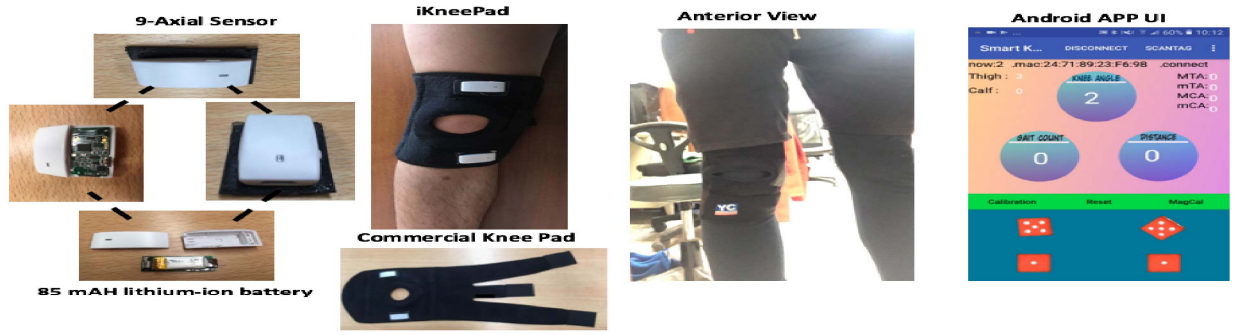
Fig. 1. The iKneePad system composed of two 9-axis sensors, sport knee pad, and Android APP.
