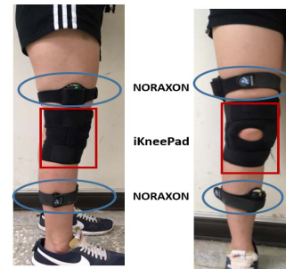
Fig. 6. The experimental setup for knee angle calculation with iKneePad and NORAXON.
